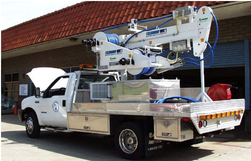
Figure 3-10 DUAL BOOM WATER QUALITY SAMPLING VEHICLE
