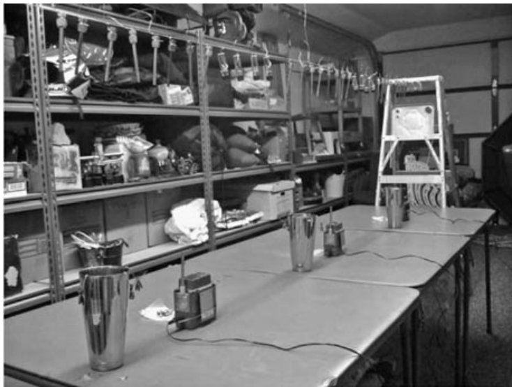
Exhibit 2. Study layout showing the three stations, various passive diffusion devices and daily active measurement with pump (note the cords to the pumps and the tubes attached thereto)
