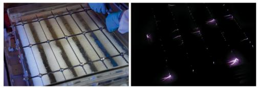
Credit: Courtesy of Selma Mededovic Thagard A plasma reactor (left) developed by researchers at Clarkson University zaps PFAS with plasma (right) to break down the molecules.
